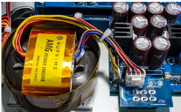
A specially customized R-Core transformer and 26000uF of filtering capacitors used in the power supply ensures that the circuitries are provided with fast and stable power.
