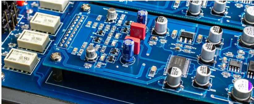
The input stage utilizes Ultra-High Bandwidth (communications applications), Low-Noise JFET for the  $1M\Omega$  input impedance circuitry. Amplification circuitry uses a Single-Ended, Non-Negative Feedback Class A module for a wide frequency bandwidth and rich second order harmonics.
