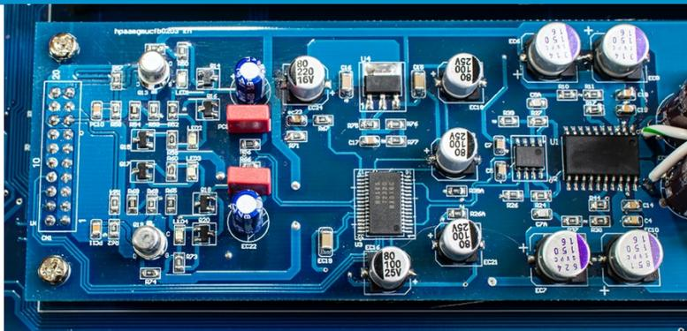
Fully balanced amplification that consists of independent circuitries for input, volume, amplification and power output stages. The volume control uses two MUSES72320 to achieve a fully balanced 100 levels (0-99) of volume adjustments. This is the best volume control we've put into a product and likely the best for any headphone amplifier.
